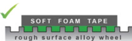
The soft foam Lohmann tape sticks better on alloy rim surfaces increasing the bond strength.
